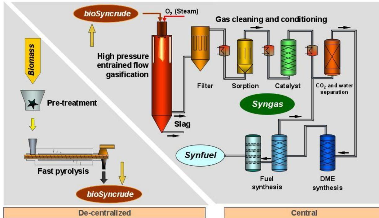
1 ton/hr gasifier of the bioliq® Process at Karlsruhe Institute of Technology operated at 30 bar for subsequent FT synthesis or at 80 bar for DME synthesis
